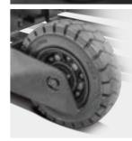
The front wheels are equipped with deep groove rubber tires, with large ground clearance, wear resistance and durability, and good shock absorption effect
